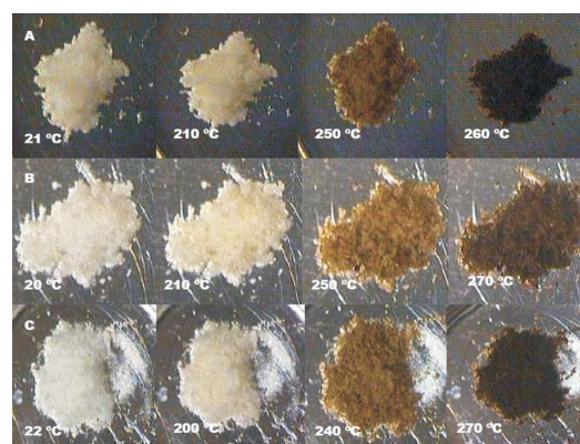
Fig. 3 DSC photovisual of croscarmellose sodium samples without water: A – CRC01 samples, B – CRC02 samples and C – CRC03 samples
